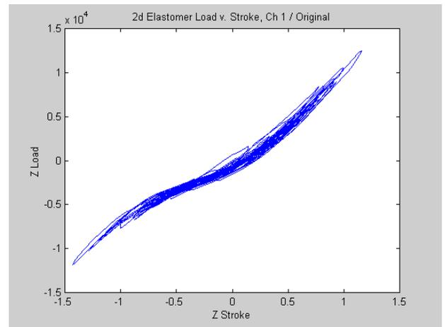
Figure 4.15 Bushing Force-Displacement, Original Lab Data, z axis
