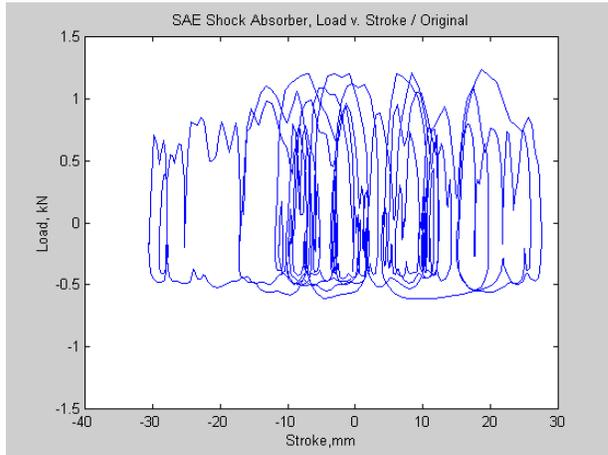
Figure 4.5 Shock Absorber #2, Force-Displacement, Original Lab Data
