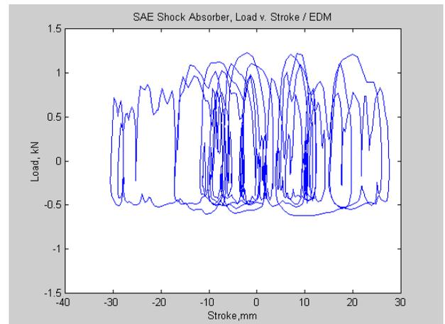
Figure 4.7 Shock Absorber #2, Force-Displacement, Empirical Dynamics Model
