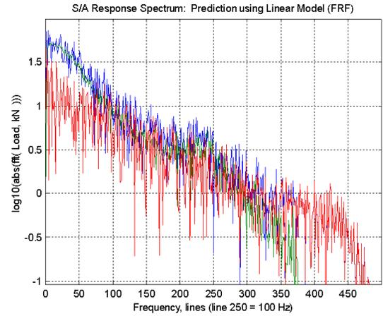
Figure 4.10 Shock Absorber #2 FFT's, FRF Model
