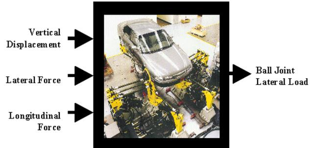
Figure 4.30 3x1 Blackbox Model for Ball Joint Strain
