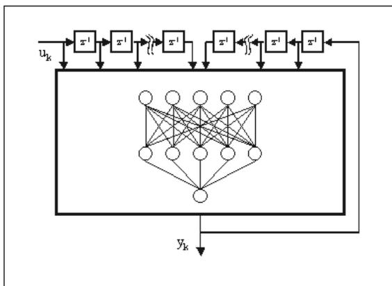
Figure 3.6 Tapped Delay Structure for Neural Net Input
