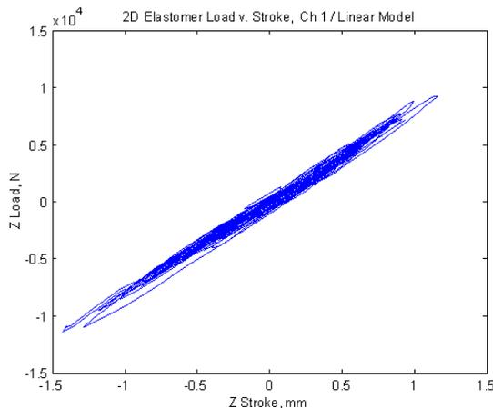
Figure 4.21 Bushing Force-Displacement, FRF Model, z axis
