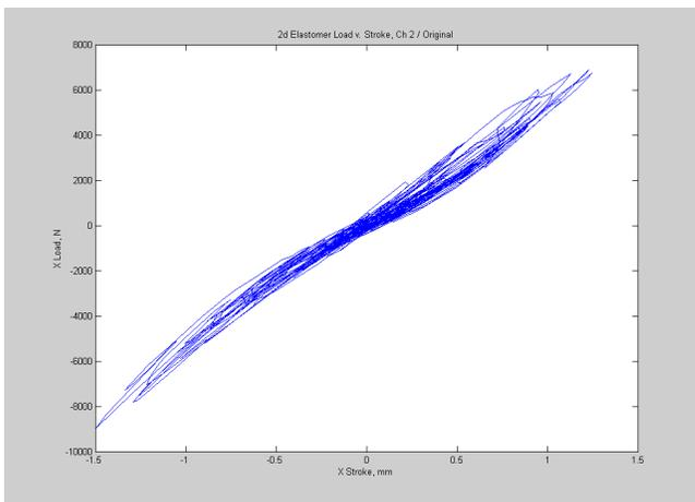
Figure 4.16 Bushing Force-Displacement, Original Lab Data, x axis
