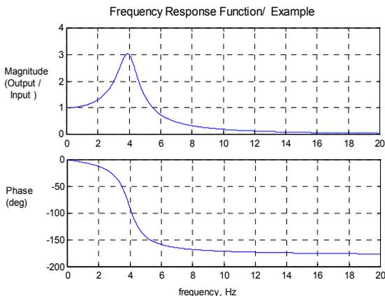
Figure 2.3 Frequency Response Function (FRF)
