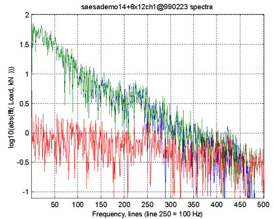
Figure 4.11 Shock Absorber #2 FFT's, Empirical Dynamics Model
