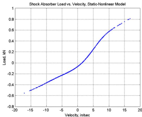
Figure 4.2 Shock Absorber #1 Force-Velocity, Polynomial Model
