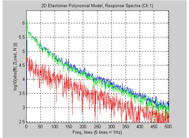
Figure 4.27 Bushing FFT's, Polynomial Model, z axis
