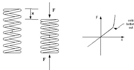
Figure 5.4 Coil Spring
