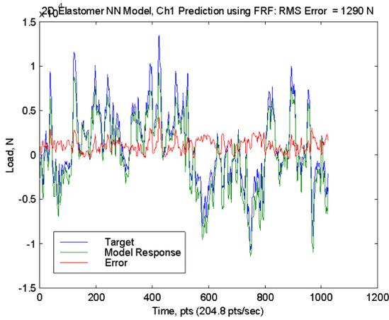
Figure 4.25 Bushing Time Histories, FRF Model, z axis
