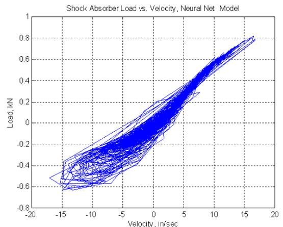
Figure 4.4 Shock Absorber #1 Force-Velocity, ED Model
