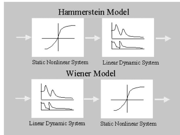
Figure 2.12 Wiener and Hammerstein Nonlinear Systems
