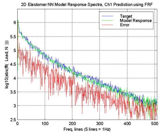
Figure 4.28 Bushing FFT's, FRF Model, z axis
