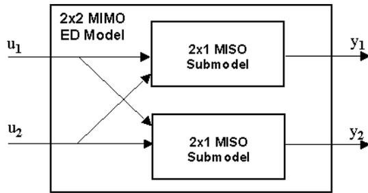
Figure 4.19 Double MISO Structure for Empirical Dynamics Model
