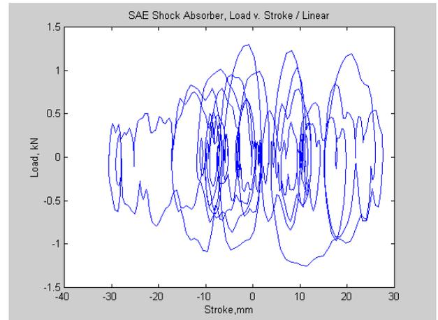
Figure 4.6 Shock Absorber #2, Force-Displacement, FRF Model
