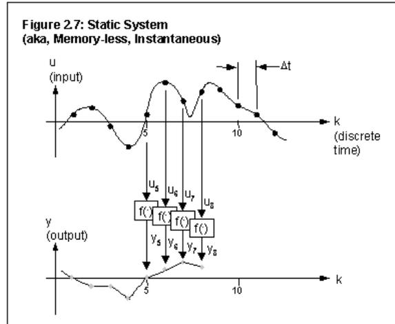
Figure 2.7: Static System (aka, Memory-less, Instantaneous)
