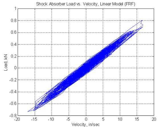
Figure 4.3 Shock Absorber #1 Force-Velocity, FRF Model
