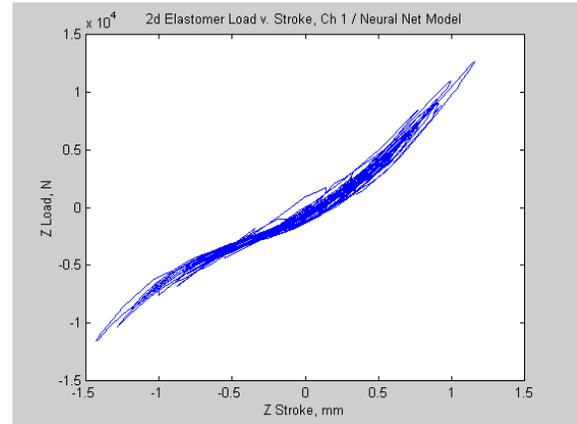
Figure 4.22 Bushing Force-Displacement, ED Model, z axis
