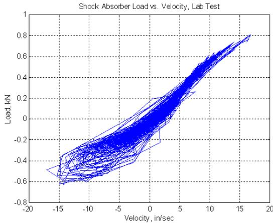
Figure 4.1 Shock Absorber #1 Force-Velocity, Original Lab Data
